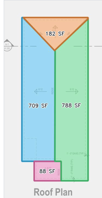
Figure 8: Current best results on held-out sheets: hip ends recovered as single triangles, main planes split exactly on the ridge, porch and garage roofs as separate planes. Every coordinate lies on a line drawn in the PDF.
