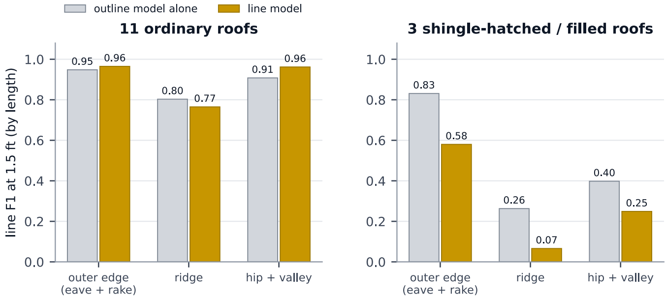
Figure 5: Roof-line F1 by class. On ordinary roofs the line model trades about four points of ridge F1 for five points of hip/valley F1 and two of outer edge; on hatched roofs it is worse on every class.
